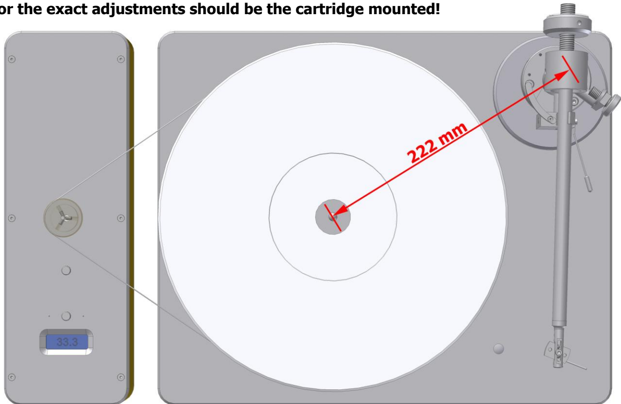
Picture 3: Distance from pivot to stylus
