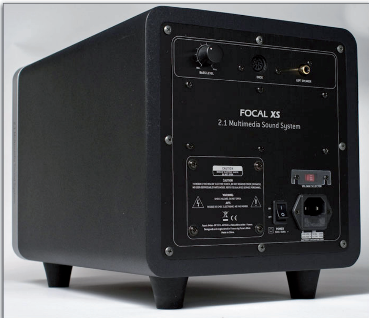
The rear of the Focal XS subwoofer has the necessary inputs and the bass level control. I set mine at a shade past 12 o'clock.
