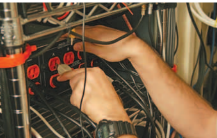
A Seemingly unafraid that a snake might be living back there, Darryl plugs components in his rack into the Furman power conditioner.
