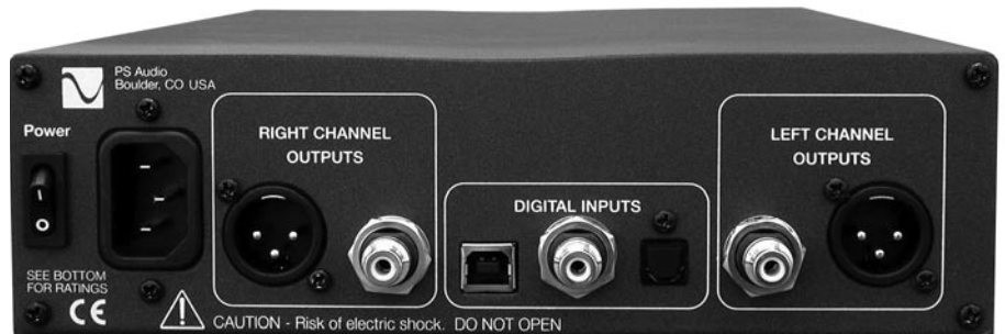
PHOTO 2: Rear view of the Digital Link III. The DAC has three digital inputs: S/PDIF coax, Toslink optical, and a USB interface for computer connection.
