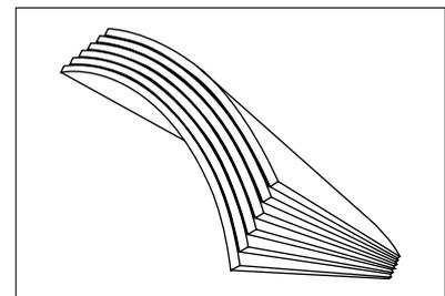
The curved HDF bended panel is made up of six 3mm MDF layers bonded by resin : this sandwich structure is naturally rigid and prevents vibration spreading by using different density layers, so as to get a reasonably flat low frequency response.
