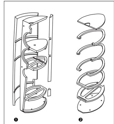
❶ Split view of Profile 918. Both HDF bended shells close in on the back bone . Notice the internal structure elements which further reinforce the loudspeaker rigidity.
