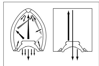
On a regular loudspeaker, the back wave generated by the driver hits the back panel and bounces back through the cone (with a very slight decay) which causes undesirable resonance. With Profile, that wave is dispersed through the loudspeaker.
